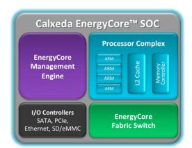
conventional CPU because its single package design enables it to run its own operating system and applications. It includes everything you need to build a complete working server.
